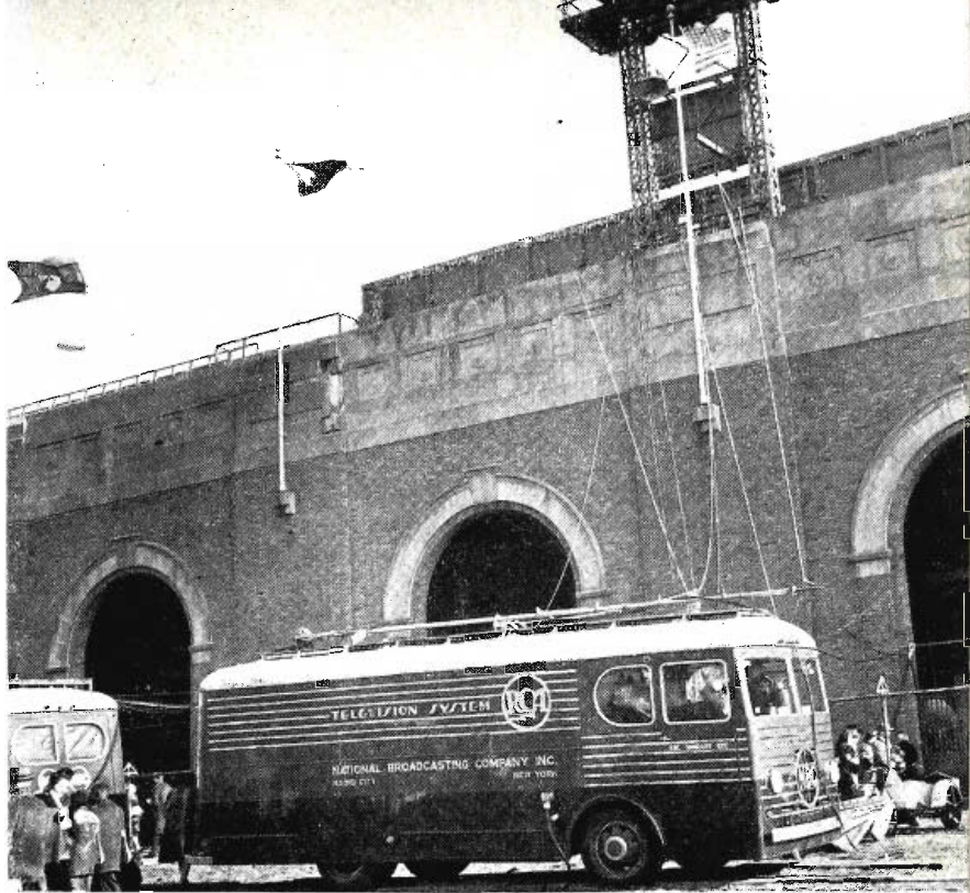
Two completely equipped RCA trucks were used for televising the Army-Navy game over WNBT. Three cameras were employed
